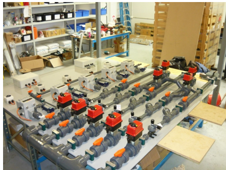
WestWater designed and manufactured a 5 train system in the Loganholme factory, it was then transported to site and installed over a day period and commissioned on the 3rd day.
