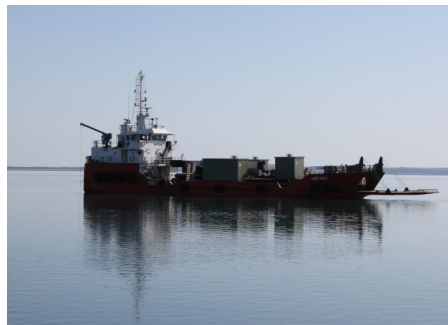
1 x Barge loaded with 3 x 20T buildings 1 x 150T crane 2 x prime movers and every nut bolt and pipe length required for the installation.
